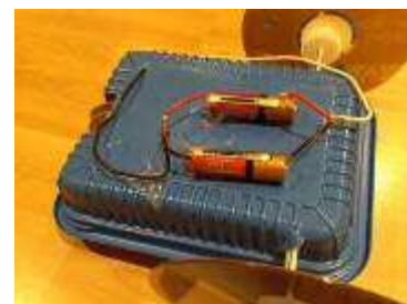
Wires connected for a parallel circuit.
