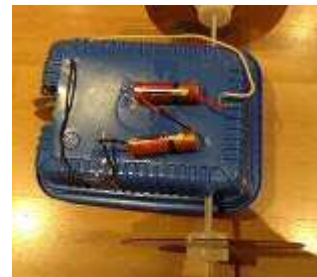
Wires connected for a series circuit.
