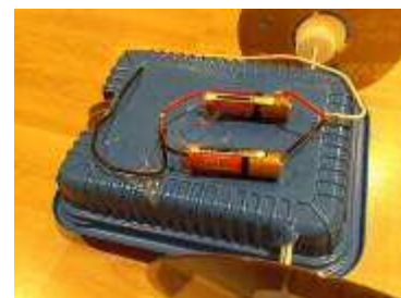
Wires connected for a parallel circuit.
